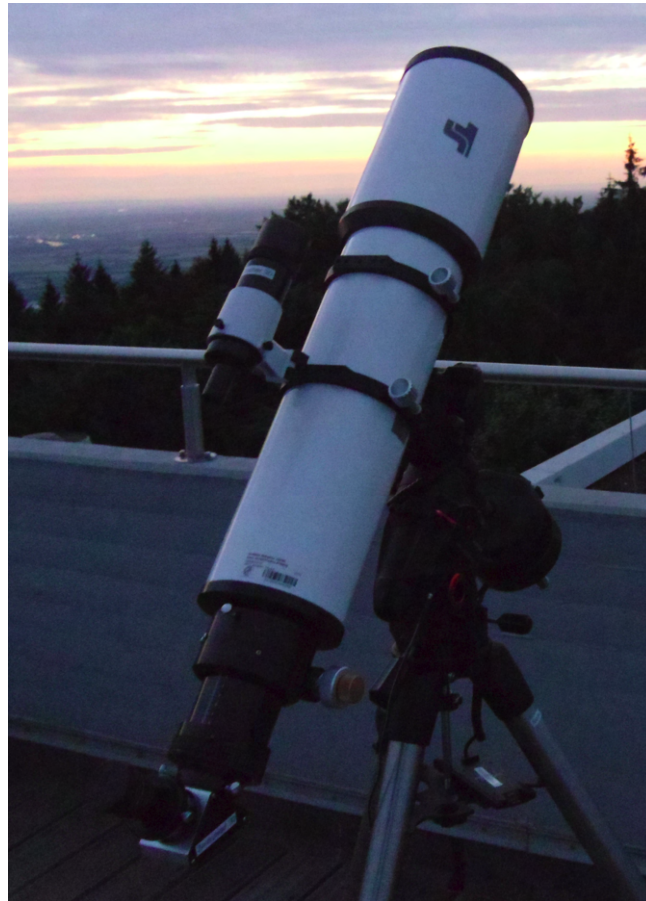
Figure 5.2: LAT undergoing testing at MPIA. The test mount, finderscope, and eyepiece pictured were later removed in the final set-up
