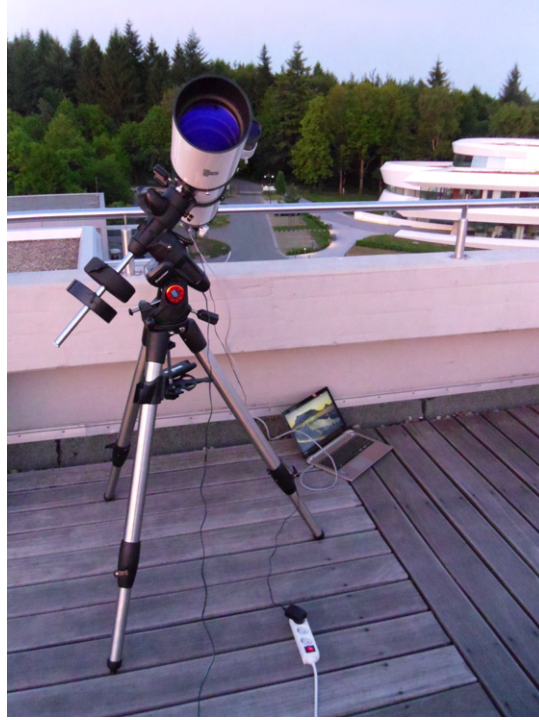
Figure 7.2: Initial calibration and testing of ProtoLAT with the Celestron mount on the roof of the MPIA. Note that the counterweights attached to the chrome bar on the left side can be adjusted in addition to the LAT position's on the mount in order to achieve balance for more precise tracking of the celestial sphere.
